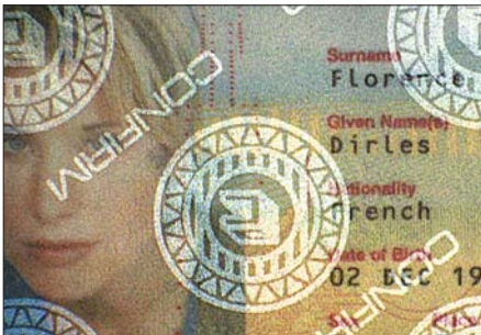
Coaxial lighting reveals retro-reflective features
