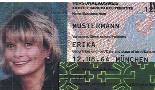
Coaxial lighting reveals retro-reflective features
