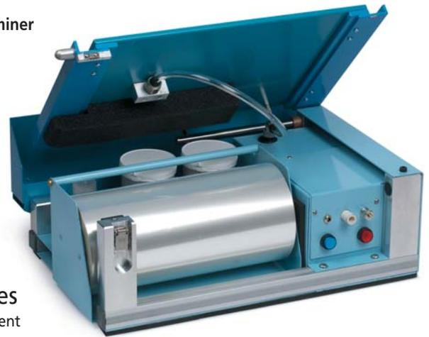
*The imaging film and developers are safely located under the vacuum bed for compact transportation. ESDA®-Lite is quickly operational by simply attaching the imaging film roll onto the locating pins.*
